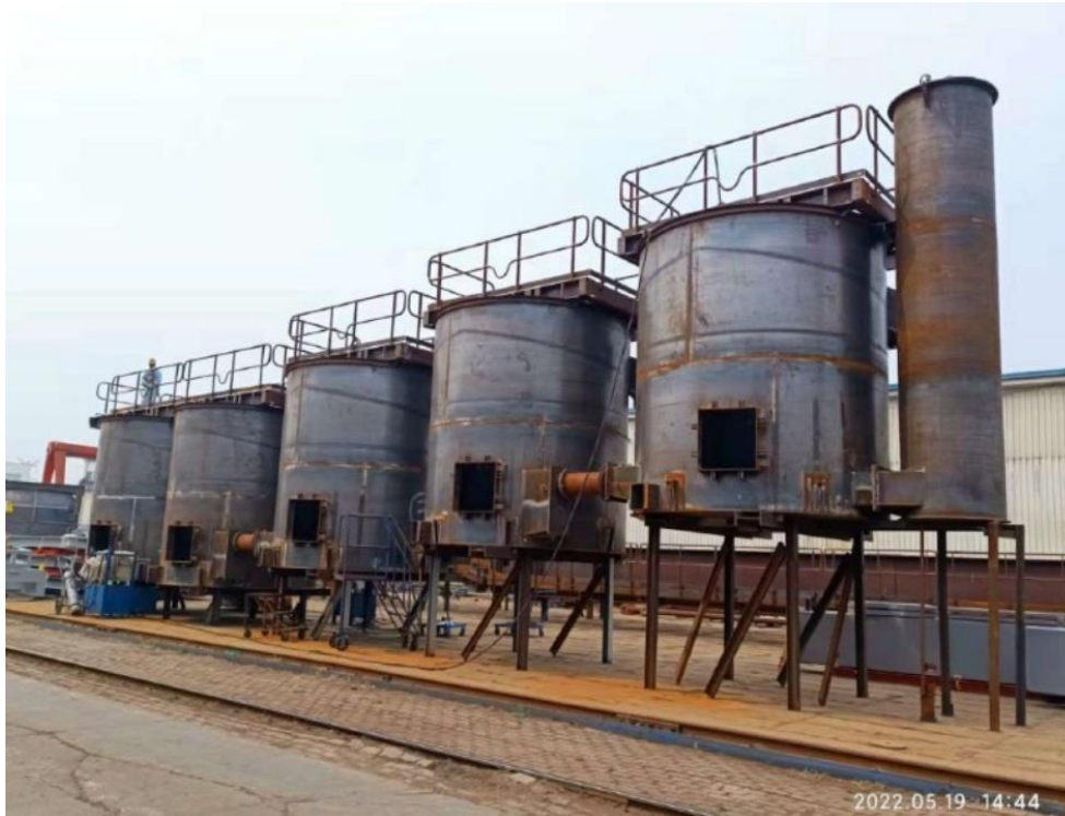
Figure 10 – Flotation cell trial assembly.
