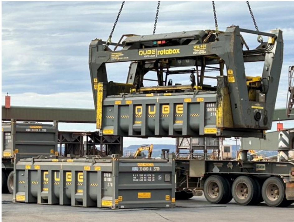
Figure 6 – Closeup view of the Rotabox™ system at work with the lifting and transfer of concentrate to the ship hold. Once inside the ship hold, the lifting mechanism rotates the container to place the concentrate in the hold (Photo 24 March 2023).
