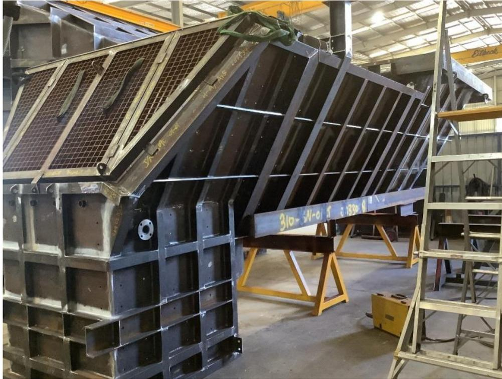
**Figure 8. Primary crusher feed chute fabrication (Perth).**
