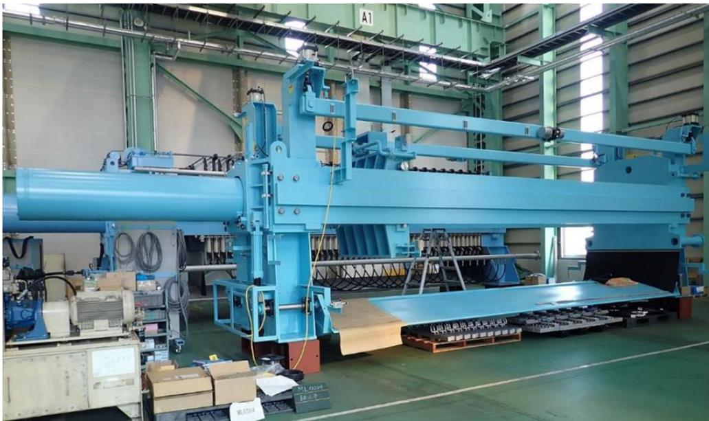
**Figure 9. Concentrate plate filter (Ishigaki) ready for shipping to Abra (Japan).**
