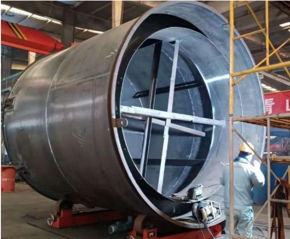
Figure 9 – Flotation cell fabrication.
