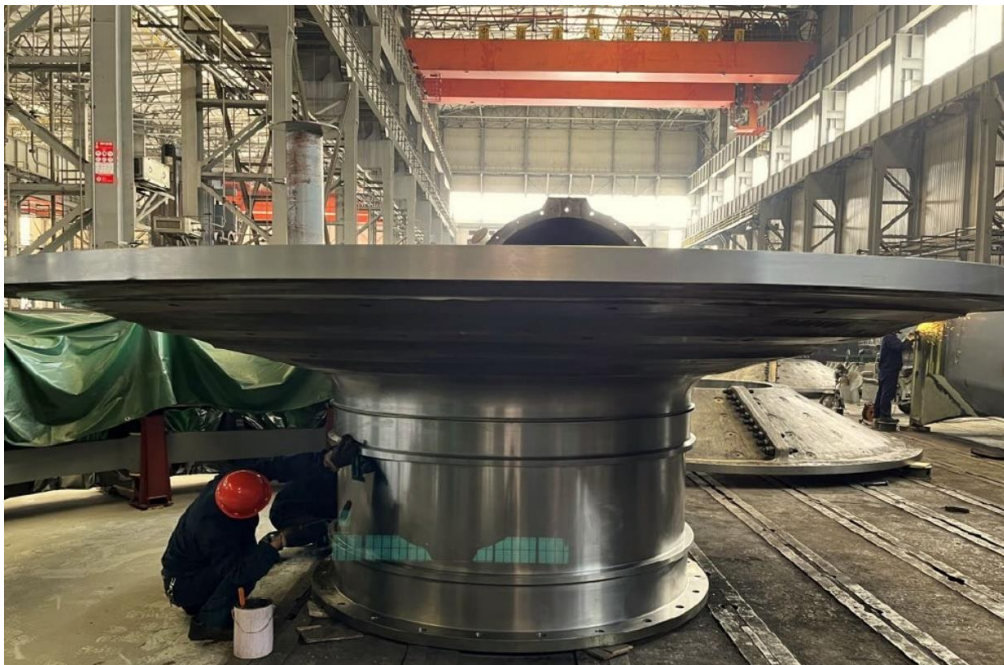
Figure 10 – Ball mill head end nearing completion.
