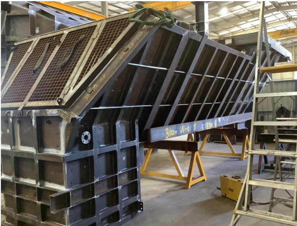
Figure 8 – Primary crusher feed chute fabrication in Perth.
