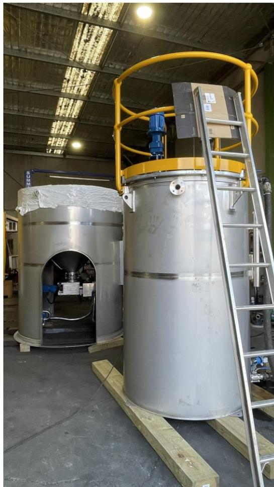
**Figure 6** – Flocculant mixing plant fabrication.
