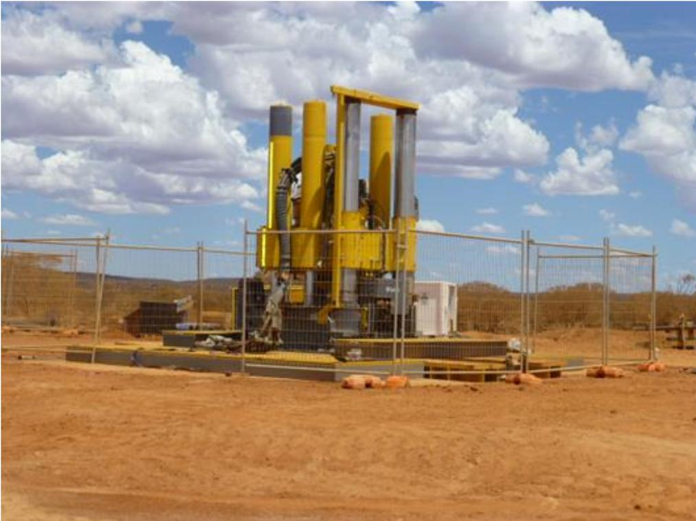
**Figure 7** – Positioning of raise drill rig on the first underground ventilation rise (4.5m diameter).
