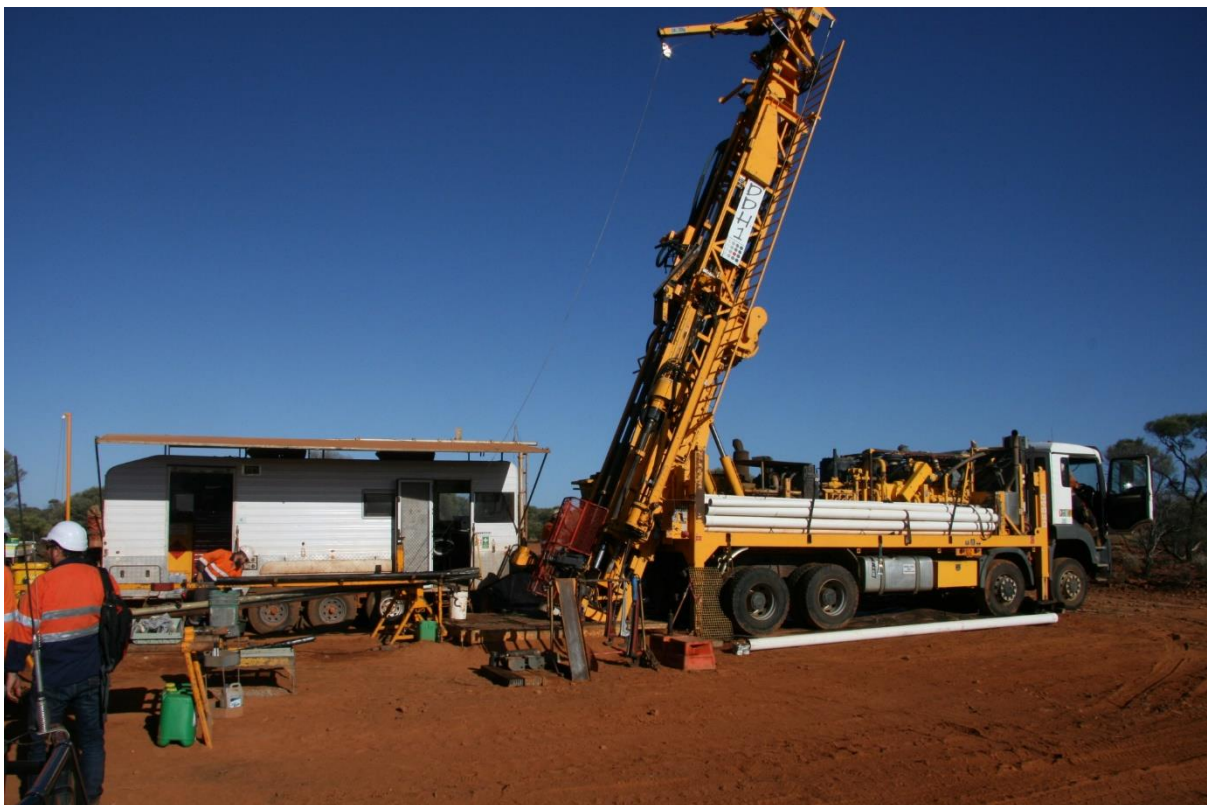
Figure 3: Diamond core drilling of Galena's first hole at Abra (AB70).
