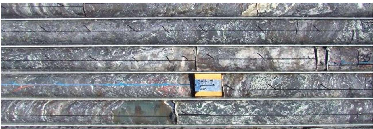
Source: GML, core from diamond drill hole AB43, approximately 351m to 356m downhole, intersections reportedly averages 8.88% Pb
