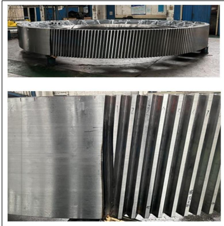
**Figure 11** – Damaged girth gear requiring replacement.
