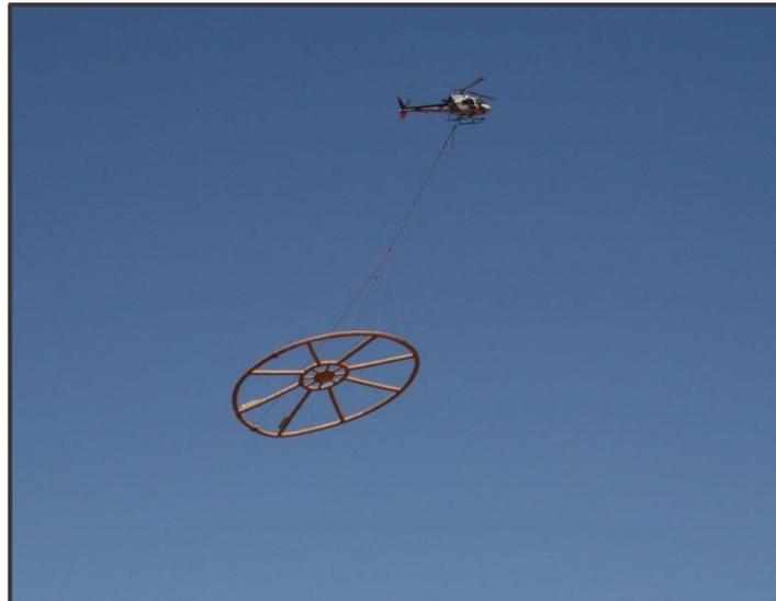
Figure 2: New Resolution Geophysics (NRG™) Australia carrying out a high-resolution helicopter hosted airborne electromagnetic (EM) survey over the Woodlands Complex
