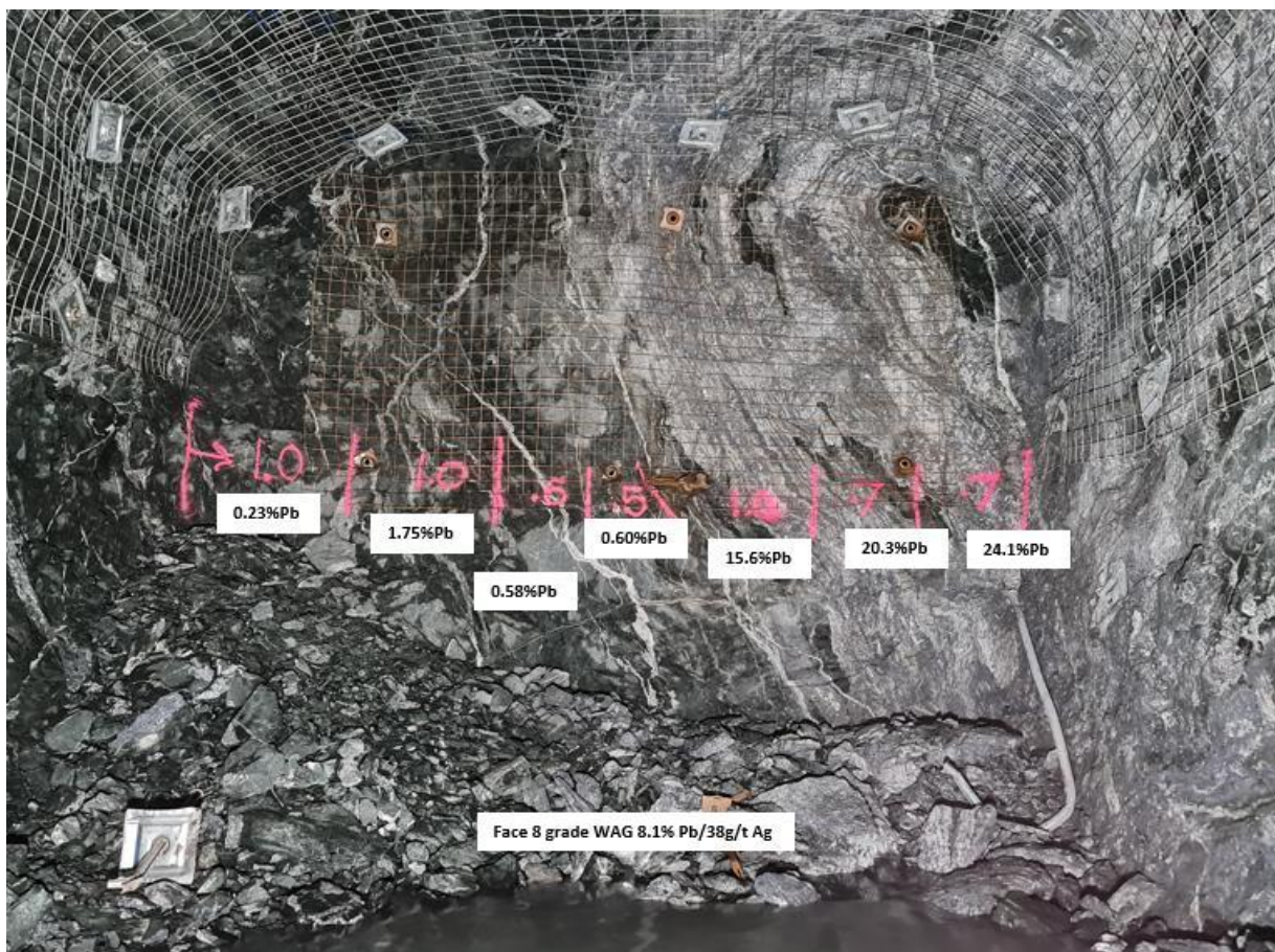
Figure 1 – Abra 1210mRL ore drive with face grades (Photo 25 January).
