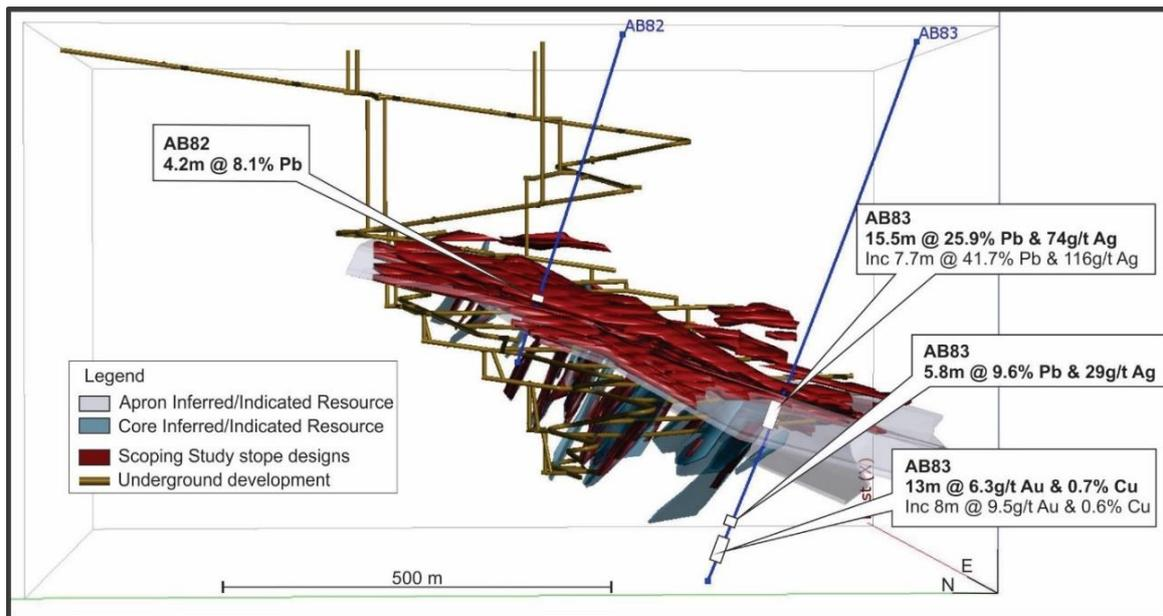
Figure 4: 3D model of the core and apron zones looking east showing AB82 and AB83, March 2018 Inferred and Indicated Resources outlines (>5% Pb wireframes) and scoping study underground mine development and stopes.
