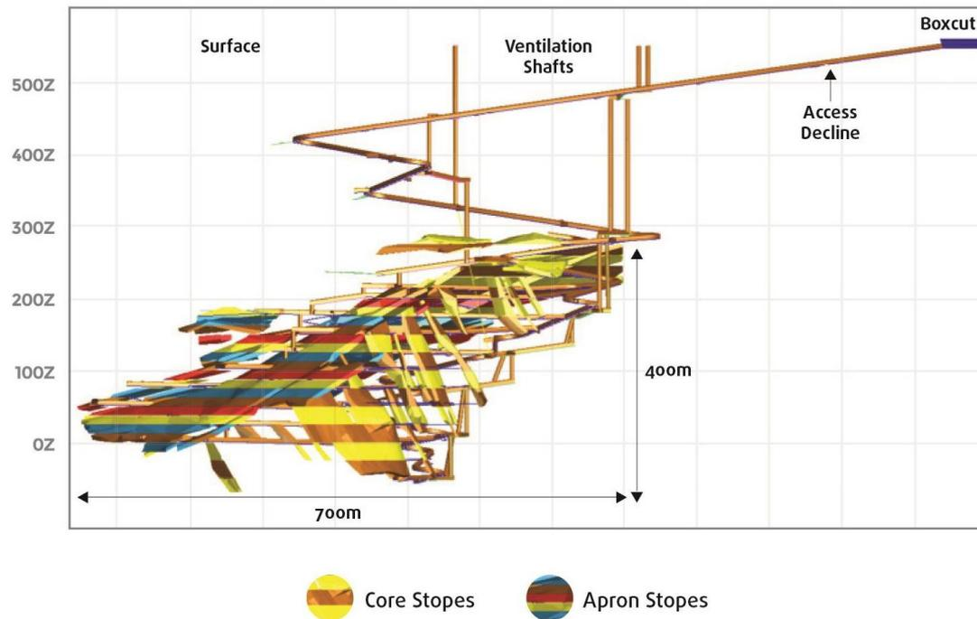
Figure 1: Abra's Conceptual Mine Design – Long Section View
