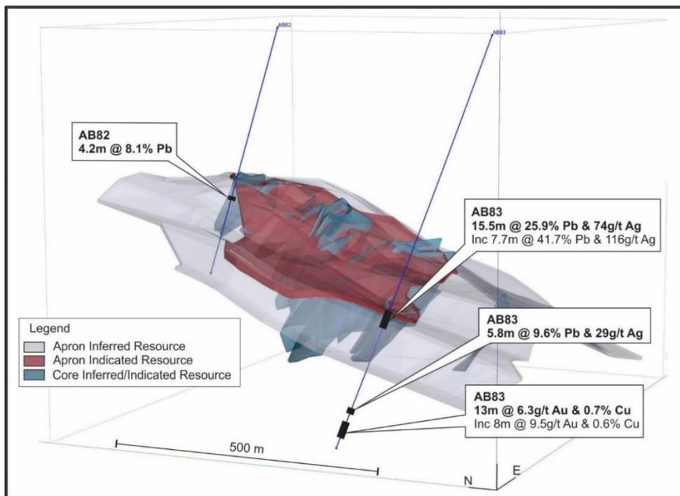
Figure 3: 3D model of the core and apron zones looking east showing AB82 and AB83, March 2018 Inferred and Indicated Resources outlines (>5% Pb wireframes).
