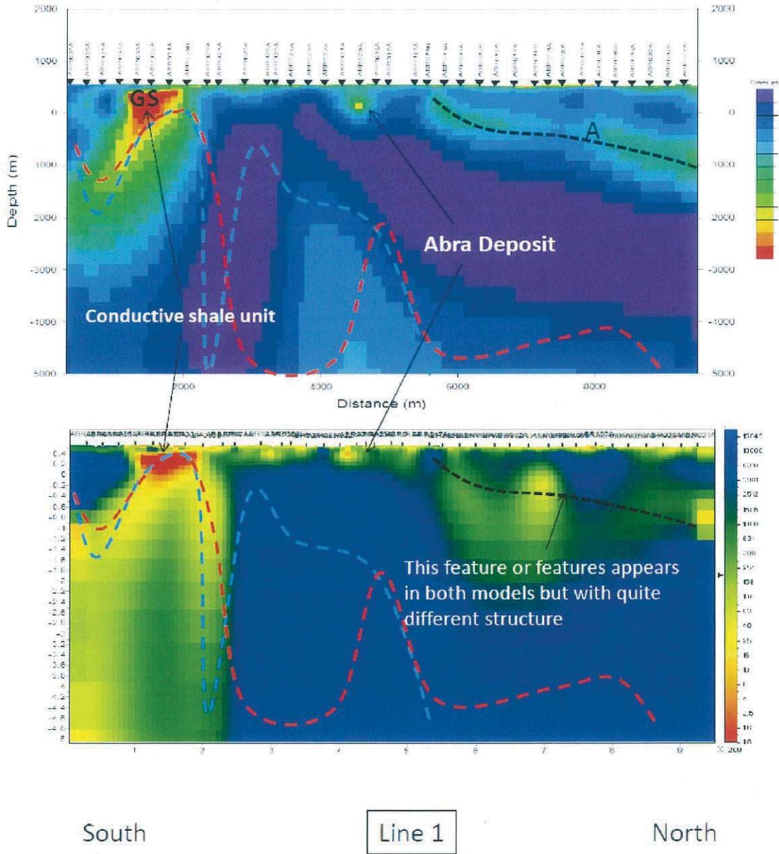
Figure 4 - North-south MT/AMT Line over Abra
