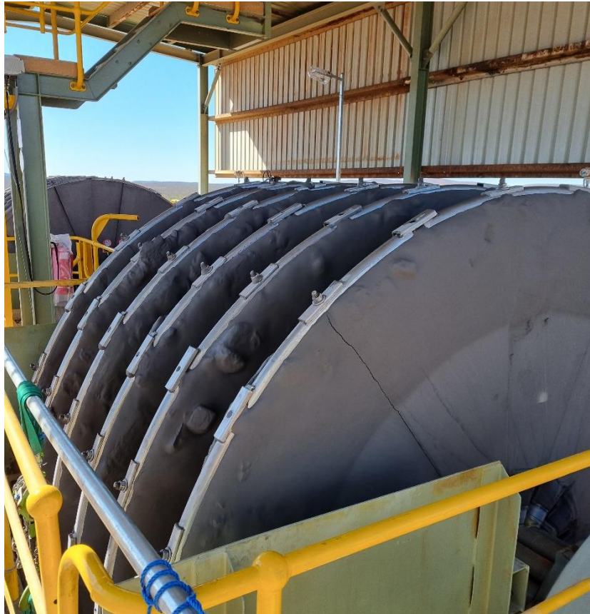
Figure 8 – Disc filters at Abra paste-fill plant dewatering the tailings prior to the paste mixing process (Photo 5 September 2023).
