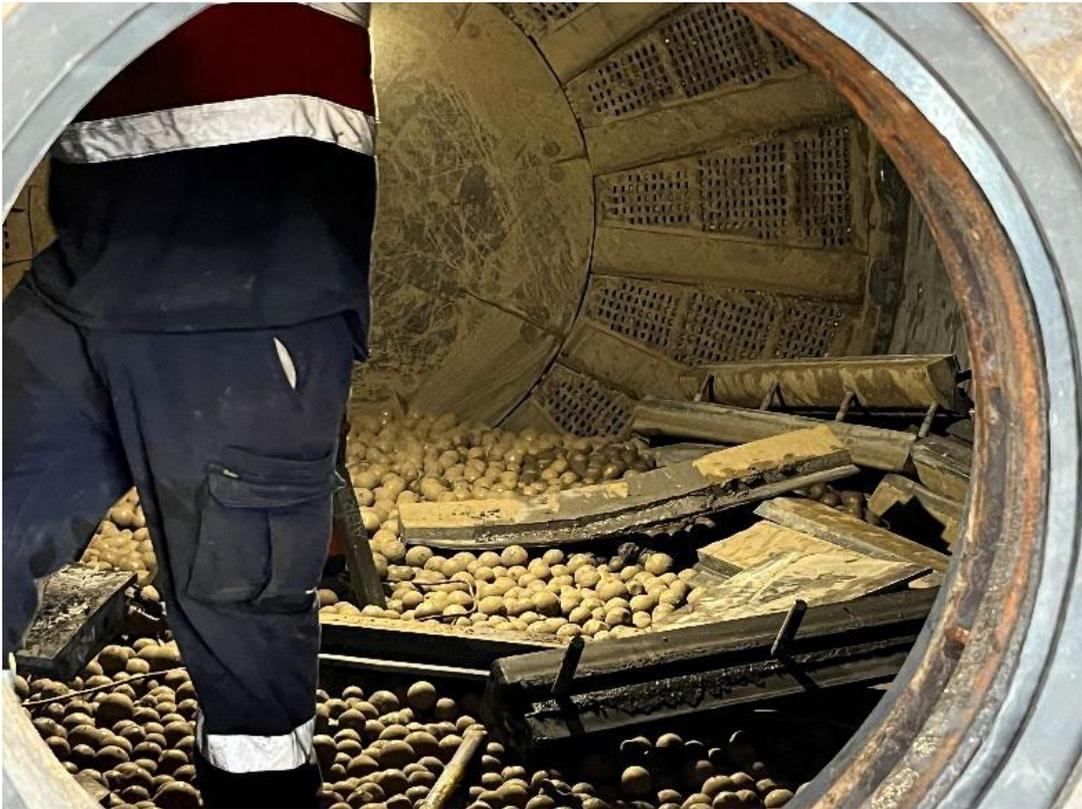
**Figure 9 – Picture taken of the inside of the mill showing removal of old liners prior to installation of the new liners (March 2024).**
