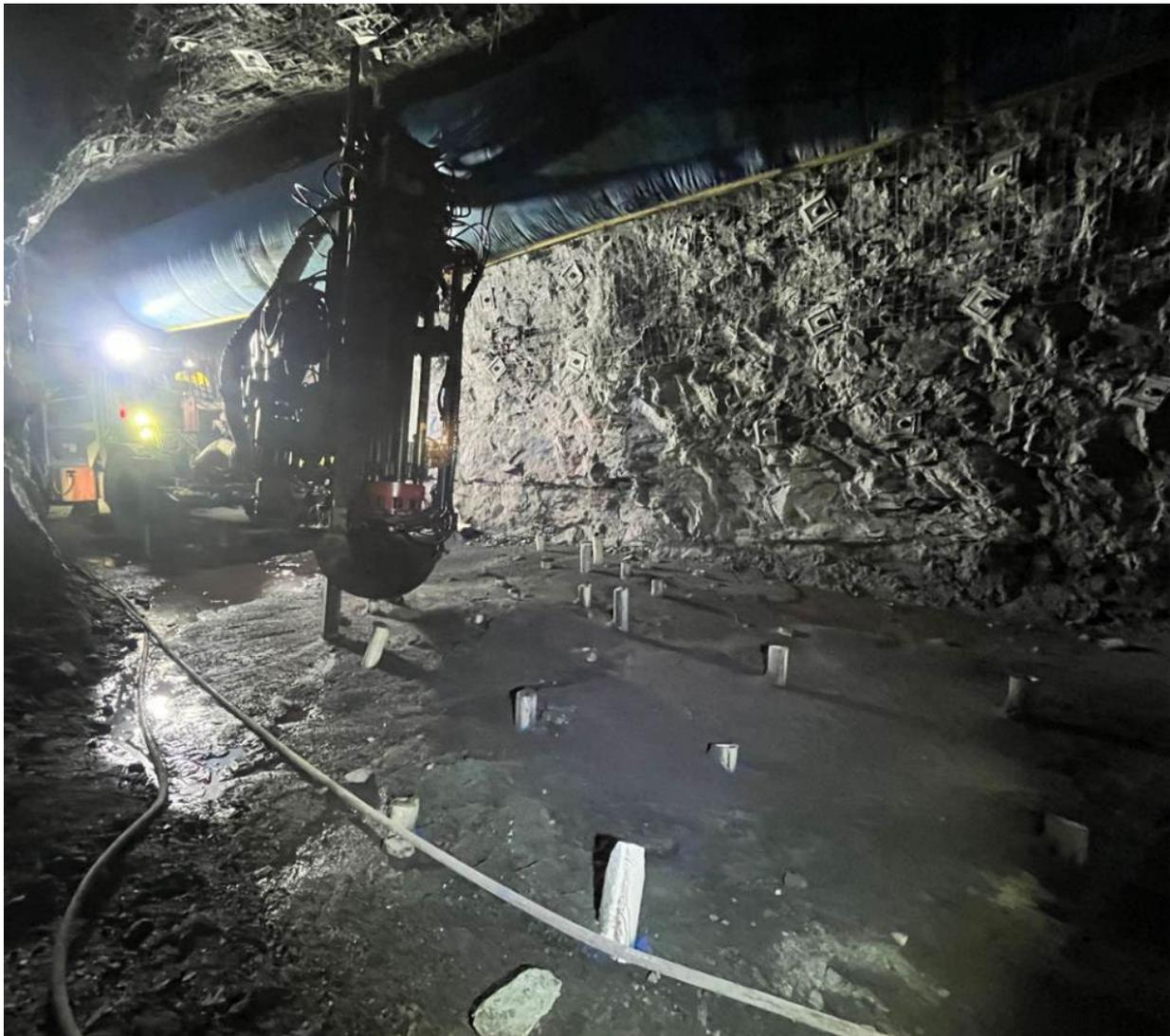
**Figure 8 – Picture showing stope production downhole drilling from AD\_1260E\_OD31 into AD\_1210\_AC2\_OD2 stope (Photo 23 March 2024).**
