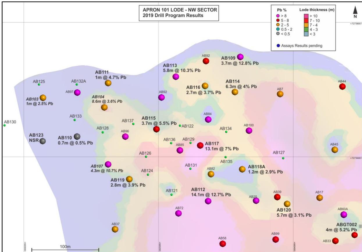
**Figure 5: Plan view of the Apron Zone 101 Lode showing drillhole pierce points (coloured by lead grade) and lode thickness contours. (N.B. thickness contours include visual thickness estimates from logged mineralisation for holes with pending assays)**
